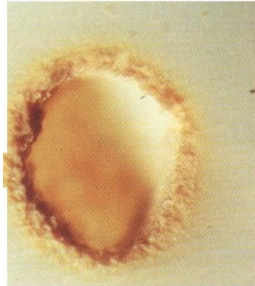
WIITH WATER DRI.Y Pr J1.0 Brownish rims as thermal side effects
